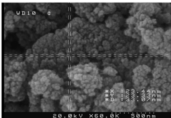
Figure 2. The SEM image of \text{Fe}_3\text{O}_4@SiO_2\text{-Im@[MnT(4-OMeP)P]} .
